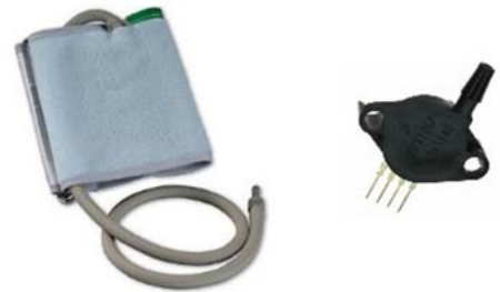
Fig. 1: Pressure cuff (left) and MPX2050GP sensor (right).
