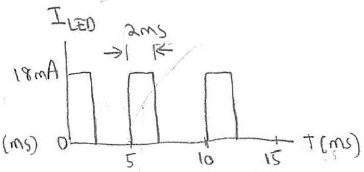
⑥ Q<sub>S</sub>: Instantaneous  $P = (0.018A)^2 (5.9\Omega) = 1.9mW$
