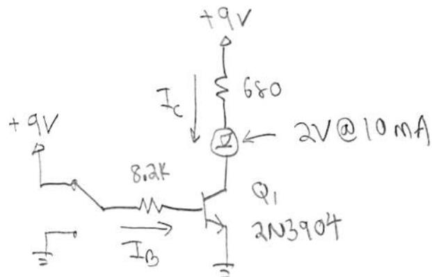
$$9 - I_B (8.2k) - V_{BE(sat)} = 0 \rightarrow I_B = \frac{9 - 0.75V}{8.2k} = 1.01 \text{ mA} \sim 1.0 \text{ mA}$$
