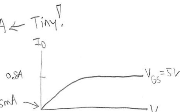
(d) IRFD9020:  $\boxed{\text{Max } V_{GS,TH} = -4V}$ (e) Q<sub>2</sub> is OFF  $\rightarrow$  Q<sub>3</sub> has  $V_{GS} \approx 15 - 15 = 0V$   $\leftarrow$  Much more positive than -4V, so Q<sub>3</sub> is OFFQ<sub>2</sub> is ON  $\rightarrow$  Q<sub>3</sub> has  $V_{GS} \approx 0 - 15 = -15V$   $\leftarrow$  Much more negative than -4V, so Q<sub>3</sub> is ON
