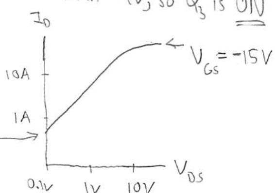
⑨ When  $Q_3$  is ON:  $R_{DS,ON} \approx \frac{1}{0.8A/0.1V} = \frac{1}{8} = \boxed{125\Omega}$
