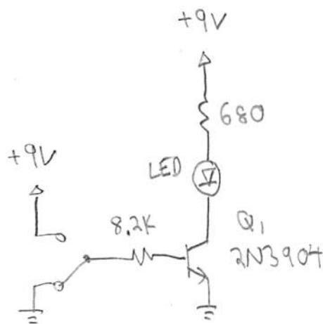
b) Switch connected to +9V:
