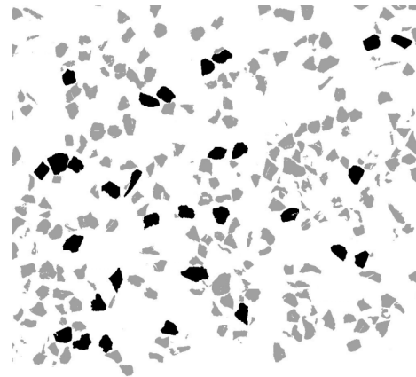
Figure 3: Processed image of crushed grains of Durango apatite showing the largest clear grain areas in black. Combining this kind of area information with the c-axis orientations from the fabric analyser produces a ranked list of candidate grains for automated fission track imaging and counting.
