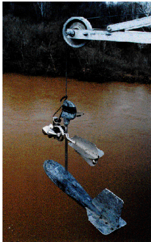
Figure 3: Current meter and weight suspended from a bridge crane (USGS, 2008).
