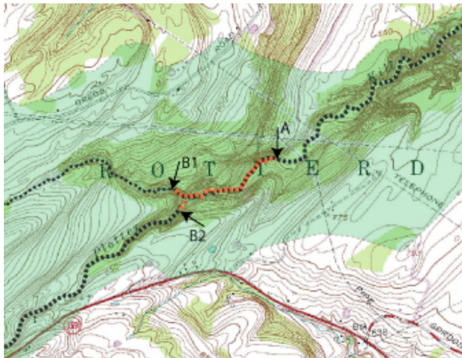
Figure 22. Estimate of the headward retreat of the knickpoint in the Plotterkill Preserve that forms the Lower Falls on Rynex Creek (B1) and on the Plotterkill Creek (B2). The knickpoint is thought to have originated in the main steep topography at point A.
