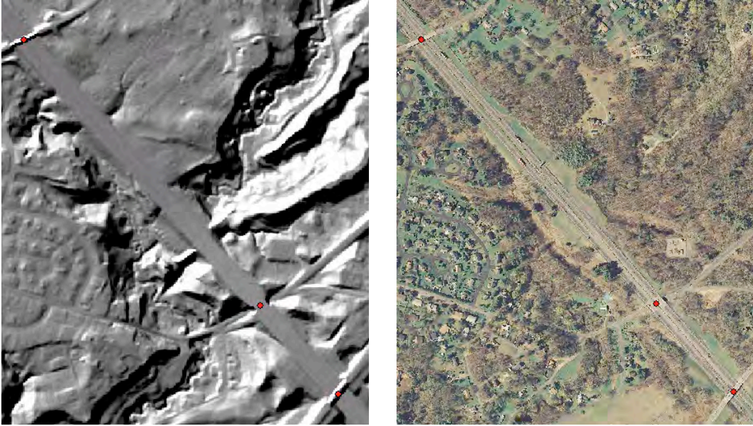
Figure 4 shows an example of elevated highways (overpasses) that were classified as ground.
