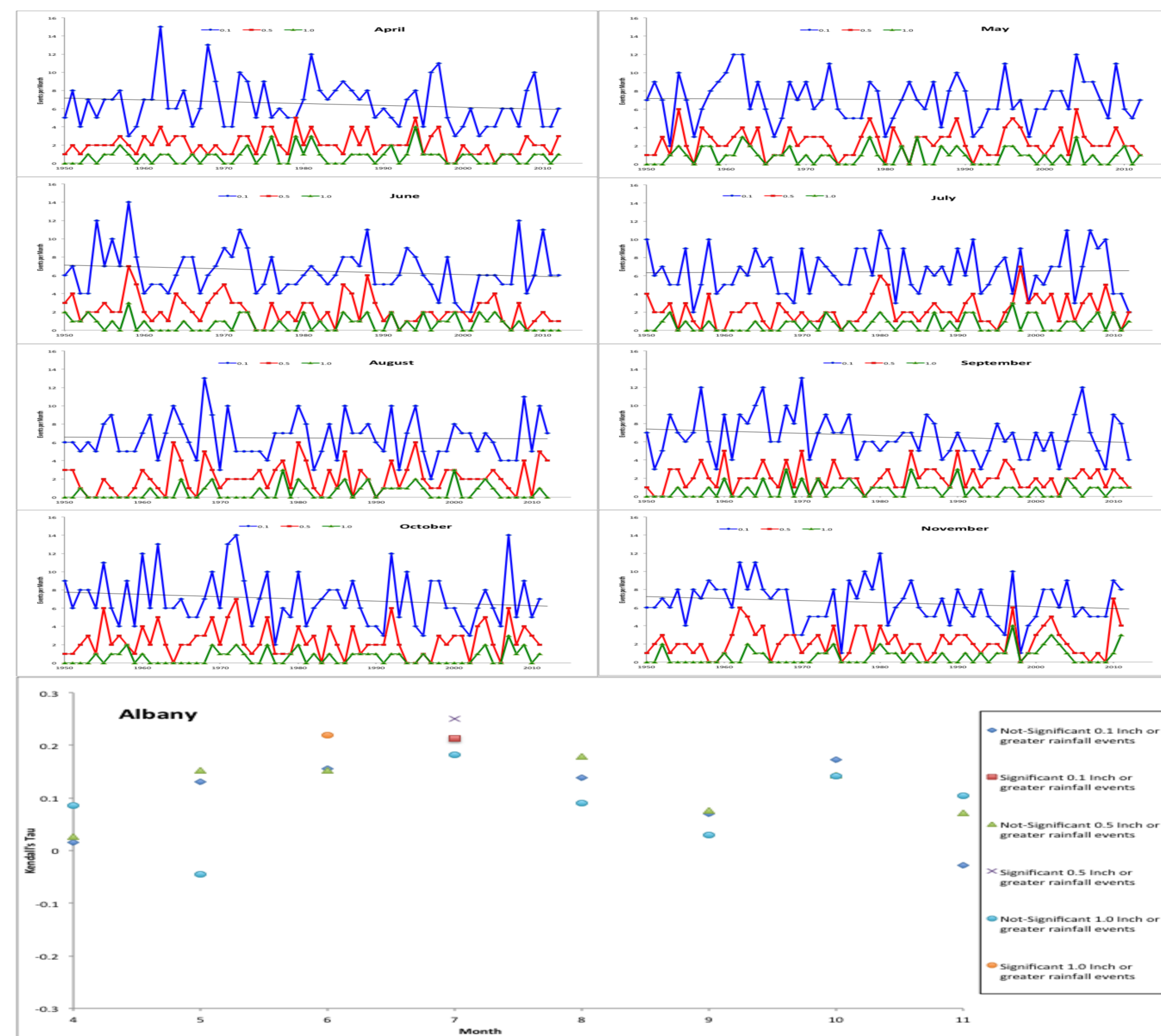
Figure 4. The top eight graphs represent rainfall events in Albany from 1950-2012. Blue lines represent 0.1 inch or greater events, red lines are 0.5 inch or greater events, and green lines represent 1.0 inch or greater events. The bottom graph represents the statistically significant or not significant rainfall event trends identified by the MK test. The results show that only June and July have statistically significant increases in rainfall events. However, overall the MK results show that rainfall and rainfall events for these defined sizes over this 62 year period are statistically increasing. This is most likely dominated by steadily increasing rainfall over the past couple decades as seen in figure 2.
