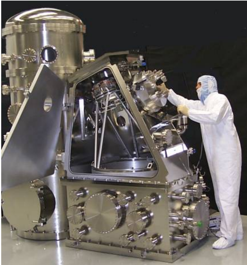
Prototype EUV exposure tool (VNL/EUV-LLC)
