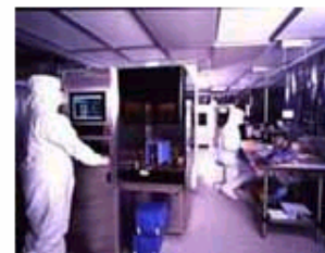
Class 10 clean room occupied with 200 mm wafer metrology
