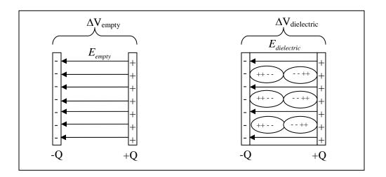
We can immediately see that the number of field lines with the dielectric is less than those without the dielectric and we define the ratio of the  $E_{empty}$  to  $E_{dielectric}$  as the dielectric constant  $\kappa = \frac{E_{empty}}{E_{dielectric}}$ , or the amount by which the number of electric field lines
