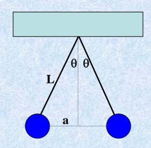
Two identical small charged spheres, each having a mass of  $3x10^{-2}$  kg, hang in equilibrium. The length of the string is 0.15m and they both make an angle  $\theta = 5^{\circ}$  with respect to the vertical. What is the magnitude of the charge on each sphere?
