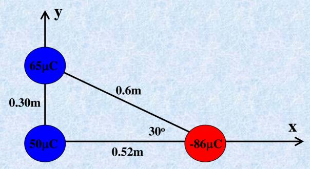
What is the net electrostatic force on the  $65\mu C$  charge due to the other two charges?
