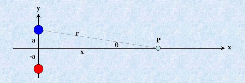
What is the electric field at a point P due to the electric dipole (two equal and opposite charges separated by a fixed distance) situated on the y-axis as shown?
