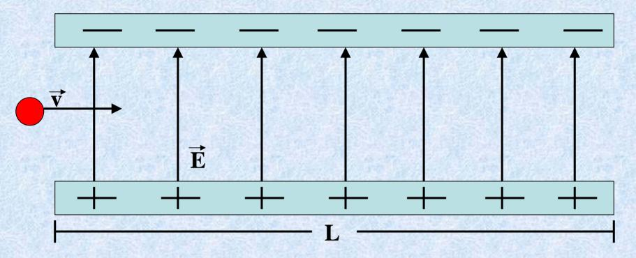
An electron enters a region of uniform electric field (E = 200 N/C) with a velocity of  $3x10^6$  m/s. What is the acceleration of the electron, the time it takes the electron to travel through the field and the vertical displacement of the electron while it is in the field? The length of the region L = 0.1m.
