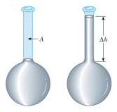
$$\Delta V = A\Delta h = \beta V_{old} \Delta T \to \Delta h = \frac{\beta V_{old} \Delta T}{A} = \frac{\frac{4}{3}\pi (0.125cm)^3 \times 1.82 \times 10^{-4} (^{o}C)^{-1} \times (30^{o}C)}{\pi (0.002cm)^2} = 3.55cm$$
