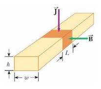
kept uncontaminated; the tube is simple to clean or cheap to replace. Two electrodes fit into the top and bottom of the tube. The potential difference between them establishes an electric current through the blood, with current density J over a section of length L. A perpendicular magnetic field exists in the same region.
