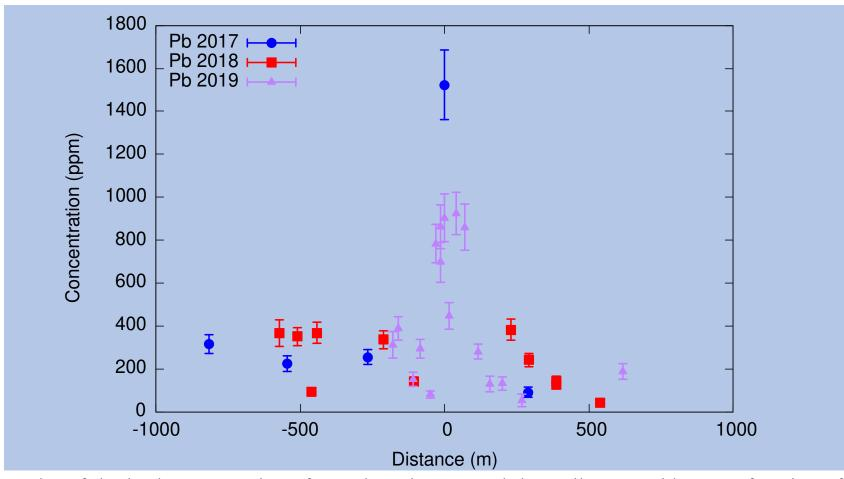
A plot of the lead concentration of samples taken around the Hell Gate Bridge as a function of distance from the bridge. The bridge is taken at zero and north of the bridge is taken as positive.
