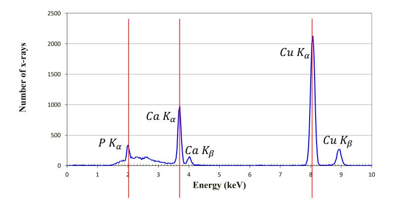
The single element standards are used to calibrate the energy scale so that we can run a real sample.
