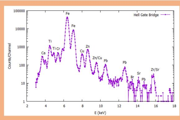
On the left, a typical PIXE spectrum for a soil sample taken near the Hell Gate Bridge, in Astoria, Queens, NY.
