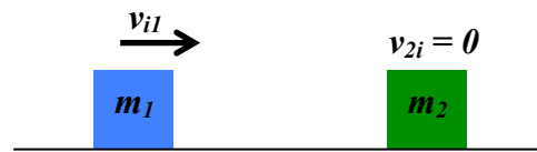
Figure 4: Mass m_1 moves to the right at an initial velocity v_{i1} and collides with mass m_2 initially at rest.
