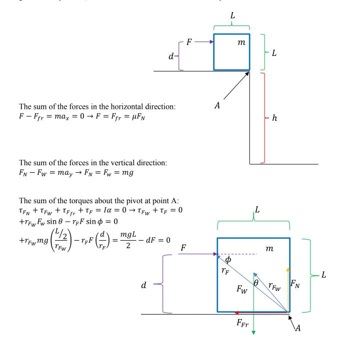
b. In terms of the quantities given in the problem, with what minimum force Fwould you need to apply to get the box to just start to tip about point A?
