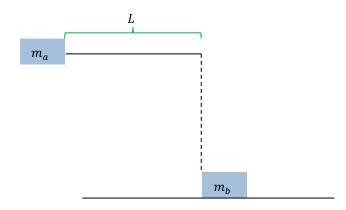
a. What is the translational speed of the block of mass  $m_a$  just before the collision? You may need that the moment of inertia of a point mass is  $I = mr^2$ .
