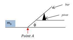
onto the bar, does the bar rotate about the pivot? If the bar rotates about the pivot, what is the initial torque about the pivot? If the bar does not rotate about the pivot, what is the reaction force on the bar at point A? Assume that  $\phi = 20^{\circ}$  and that the pivot is located at a distance of 70% of the way from point A to the end of the bar.
