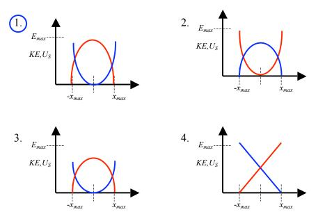
Since there's no friction, at any point the sum of the kinetic and potential energies have to sum to the total energy by:  $\Delta E = 0 = \Delta K e + \Delta U_g + \Delta U_s = (\frac{1}{2}mv^2 - 0) + (\frac{1}{2}kx^2 - \frac{1}{2}kx_{max}^2)$
