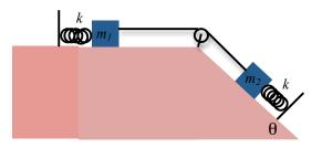
Using energy methods we have (where at maximum extension of the left spring (and maximum compression of the right spring) the velocity of the blocks being zero) and block #1 having no change in gravitational potential energy
