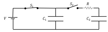
a. How much charge (in magnitude) is on each plate and how much energy is stored in the  $2\mu F$  capacitor when fully charged?
