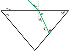
a. What is the critical angle for the topaz/air interface on the right and what is the speed of light in topaz?
