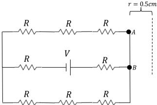
Since the resistance of the upper and lower branches are the same, the total current will split in half, with half going through the upper branch and half going through the lower branch.
