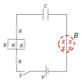
c. At a time  $t = 3\tau$ , what is the power dissipated across all the resistors in the circuit if the current is again given by  $I = I_{max}e^{-\frac{t}{R_{eq}C}}$ ?
