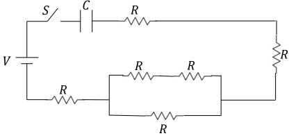
a. What is the time constant for the circuit? Hint: the capacitor is constructed out of two square plates with sides of length L = 50cm and separated by 0.5mm of air.
