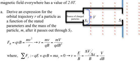
b. Suppose that you have two singly ionized isotopes of sodium,  ${}^{22}_{11}Na$  and  ${}^{24}_{11}Na$ , that are the source of charged particles, by what amount would the two isotopes be separated when they strike the detector (either one of the blue plates) if the separation between the capacitor plates is *5mm*? Will the isotopes strike the detector above or below the exit at S<sub>2</sub>?
