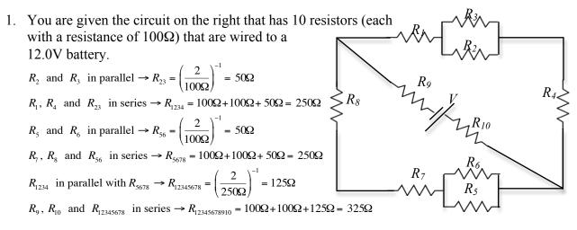
a. What are the equivalent resistance  $R_{eq}$  of the circuit and total current  $I_{total}$  produced by the battery?
