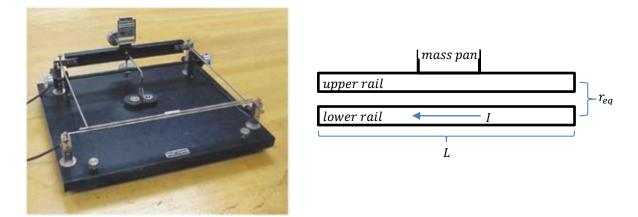
a. What is the direction of the current flow in the upper rail so that the upper rail will move up away from the lower rail? Explain your answer fully to earn full credit.
