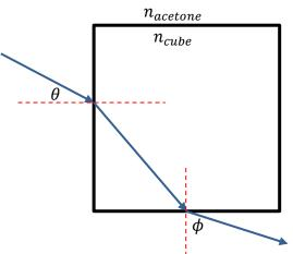
a. The light is incident on the left face of the cube at  $\theta = 65^{\circ}$  and exits the from the lower face at  $\phi = 75^{\circ}$ . What are the indices of refraction of acetone and of the cube material? Hint:  $\sin(90 - \delta) = \cos \delta$ .
