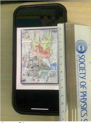
$$M = \frac{h_i}{h_o} = \frac{d_i}{d_o} \to d_i = Md_o = \left(\frac{h_i}{h_o}\right)d_o = \left(\frac{7.4cm}{99cm}\right)d_o = 0.075d_o$$
