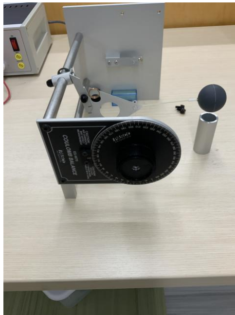
Figure 1.2: Torsion balance laid on its side with the slide assembly removed.
