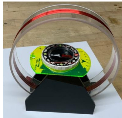
Figure 4.2: A current carrying coil of wire will produce a magnetic field perpendicular to the earth's magnetic field.
