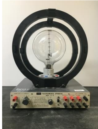
Figure 4.4: Photograph of the apparatus. The Helmholtz coils generate a uniform magnetic field that the electron beam passes through.
