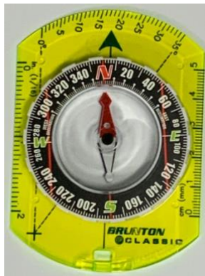
Figure 4.1: Compass points north in the earth's magnetic field.
