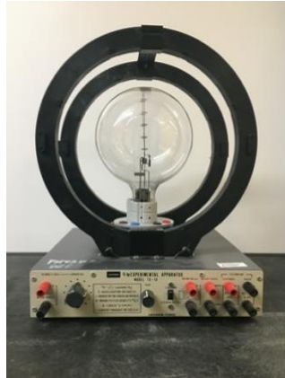
Figure 4.4: Photograph of the apparatus. The Helmholtz coils generate a uniform magnetic field that the electron beam passes through.
