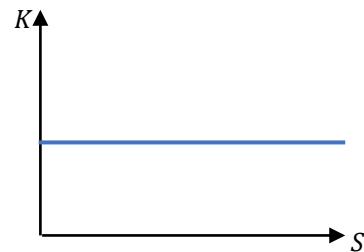
Figure 6.2: A plot of the kinetic energy of an ejected electron as a function of the intensity of light incident on a metal surface.
