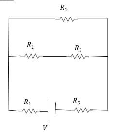
Resistors  $R_2$  and  $R_3$  are in series:  $R_{23} = R_2 + R_3 = 100\Omega + 100\Omega = 200\Omega$
