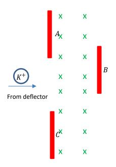
After the ions leave the deflection region only the magnetic force remains. And by since the ions experience an upward initial force and by the right-hand rule, the potassium ions will strike the detector A.
