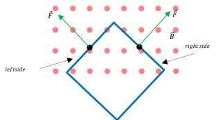
As the wire lop falls out of the magnetic field, the magnetic flux through the loop of wire will decrease. To undo the decrease in magnetic flux we need the magnetic field produced by the loop of wire to point out of the page. This produces a counterclockwise current flow.
