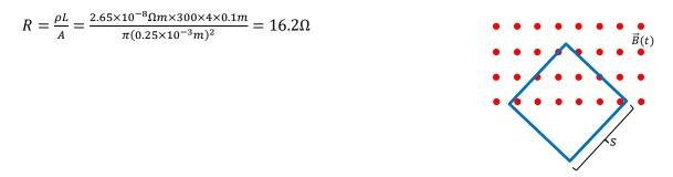
2. The wire (lying in the plane of the page) has a magnetic field pointing out through one-half of the square and the magnetic field is perpendicular to the plane of the page. The magnetic field varies in time according to B(t) = 0.437 + 0.912t, for t in seconds and B in Tesla, over a time interval  $0 \ll t \ll 10$ . What is the magnitude and direction of the induced current in the loop of aluminum wire?
