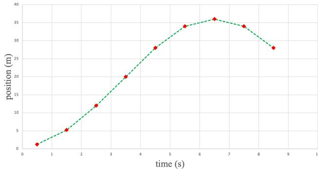
I Over the interval  $0s \leq t \leq 3s$ , the car is accelerating and its position is increasing in the positive x-direction at a quadratic rate as shown on the plot.
