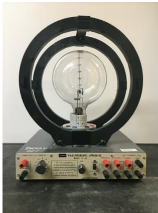
Figure 1: Photograph of the apparatus. The Helmholtz coils generate a uniform magnetic field that the electron beam passes through.
