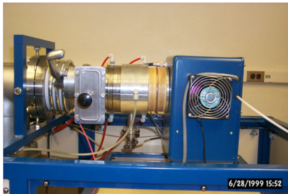
Figure 2: Low energy end of the particle accelerator, showing the ion source with the cage removed. The ion source is operational as shown by the pink glow behind the fan on the right edge. The ion source holder can also be seen in the middle of the figure below the beam line.
