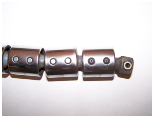
Figure 7: The Pelletron chain. The Pellets are the metal pieces the grey pieces in between each metal pellet are the insulating links.
