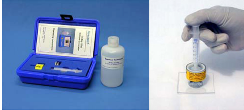
Figure 6: Cs/Ba isotope generator kit on the left. The cow is shown on the right with the syringe of the acid solution attached. The cow is milked into a pan for use in an experiment from Pasco. http://www.pasco.com/prodCatalog/SN/SN-7995_isotope-generator-kit-barium-137-m/#overviewTab
