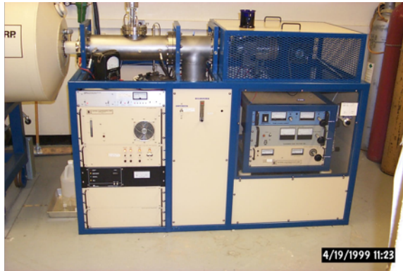
Figure 1: Low energy end of the particle accelerator, showing the ion source under a cage. The cage is to protect the operator from a static discharge when the accelerator is operating.
