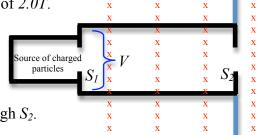
b. Suppose that you have two singly ionized isotopes of sodium,  $^{22}_{11}Na$  and  $^{24}_{11}Na$ , that are the source of charged particles, by what amount would the two isotopes be separated when they strike the detector (either one of the blue plates) if the separation between the capacitor plates is 5mm? Will the isotopes strike the detector above or below the exit at  $S_2$ ?
