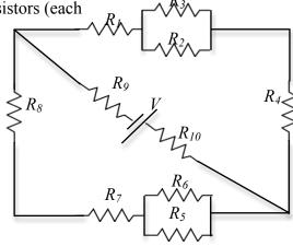
a. What are the equivalent resistance  $R_{eq}$  of the circuit and total current  $I_{total}$  produced by the battery?
