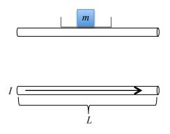
The current flowing in the bottom bar produces a magnetic field at the upper wire that points out of the page. The force on this upper wire due to the magnetic field the wire is interacting with has to point up the page to balance the downward force of the weight of the added mass. Thus by the RHR the current has to flow from *right-to-left*. To determine the magnitude of the current we examine the forces that act on the upper wire. We have:
