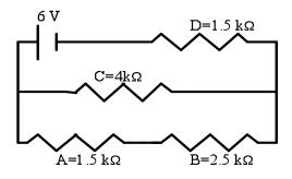
The total current produced by the battery is given by Ohm's Law
