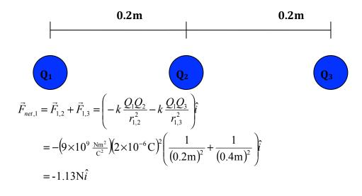
$$\vec{F}_{net,2} = \vec{F}_{2,1} + \vec{F}_{2,3} = \left( -k \frac{Q_2 Q_1}{r_{2,1}^2} + k \frac{Q_2 Q_3}{r_{2,3}^2} \right) \hat{i}$$
