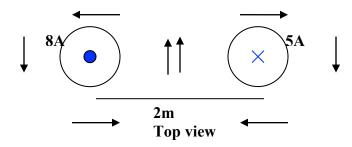
17.18 The magnitude of the magnetic force on a wire (#1) due to a current flowing in another wire (#2) located at a distance *d* away is given by  $\frac{F_{1,2}}{L} = \frac{F_{2,1}}{L} = I_1 B_2 = \frac{\mu_0 I^2}{2\pi d}$ .
