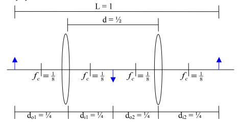
Here the magnification of the lens on the left is  $M_L = -\frac{d_o}{d_i} = -\frac{1/4}{1/4} = -1$  while the
