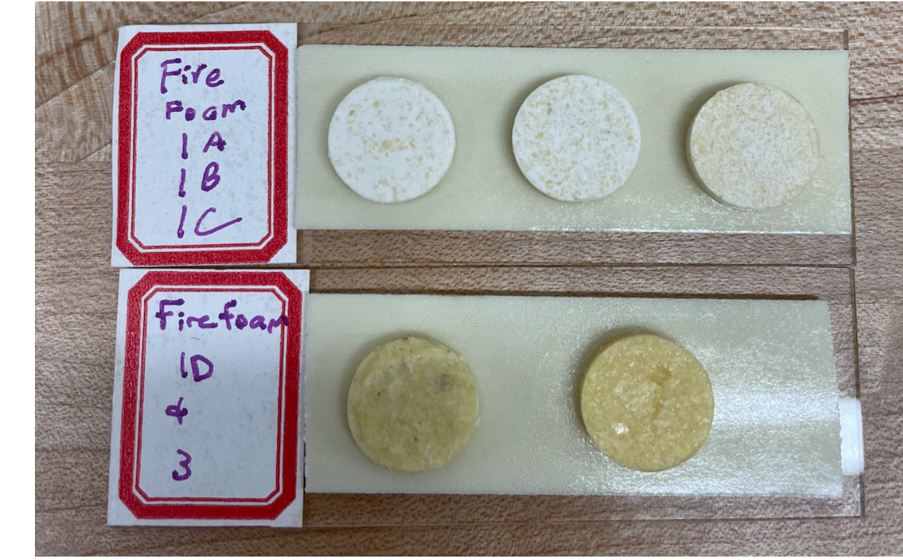
Figure 4: Firefighting foam targets of varying concentrations of NaF and cellulose binder
