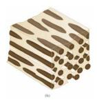
(a) Bragg's law applies to the space lattice of melanin rods. Consider the planes  $d=0.25~\mu\mathrm{m}$  apart. For light at near-normal incidence, strong reflection happens for the wavelength given by  $2d\sin\theta=m\lambda$ . The longest wavelength reflected strongly corresponds to m=1:
