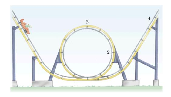
Consider a roller coaster car (with negligible friction) going around a loop of radius 20m. The car barely makes it around the top of the loop, and at the top the riders feel weightless. What is the speed of the roller coaster at the top of the loop? What is the speed of the roller coaster at points 1 and 2? What is the difference in heights between positions 1 and 4 if the speed at 4 is 10m/s?
