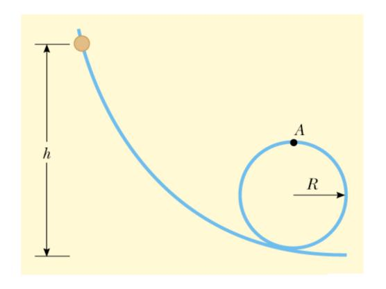
A bead slides without friction around a loop-the-loop track as shown above. If the bead is released from a height h=3.5R, what is the speed of the bead at point A? What is the normal force at A if the bead has mass 5g?
