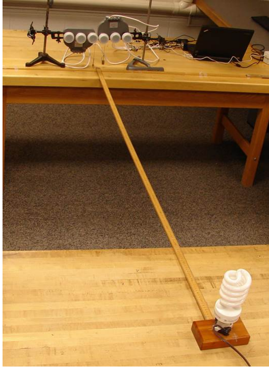
FIG. 2: Set up with the CFL in the foreground and the LNBs, connected to laptop, 2 meters away.
