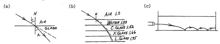
With some extra effort and a laser, you can simulate atmospheric refraction in the classroom; the experience is very rewarding. A liquid, a variable sugar solution, works well. You must establish continuous "layers" of different sugar concentrations that create a vertical gradient of indices of refraction similar to that in the earth's atmosphere.
