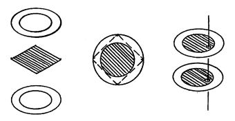
Place the pair on the OHP stage aligned and "crossed" (90°) to show the extremes of light transmission. From now on, one filter will rest on the stage while the second filter is suspended above it, leaving a space in between to work. For convenience, a lightweight (butterfly?) stand (see diagram) is recommended to hold (suspend) the second filter. It can be made out of scrap pine and plywood, a short wood dowel or Al rod, four small FH screws, and a thumb screw.
