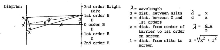
You may <u>not</u> use 1 in place of z because of the high quality of this grating.  $\theta$  is much too large (the dispersion too great). Of course, d is the reciprocal of 750 slits/mm or equal to 1/750 mm or .00133 mm between slits. x and z (1?) may be measured with a meter stick or metric tape measure. Don't expect a <u>useful</u> 2nd bright order with this grating; too much distortion.
