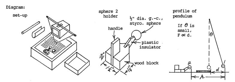
Materials: OHP, "1 cm" grid, fence, 1¢, dowel with sphere 1, holder with sphere 2, masking tape, pvc rod, wool cloth
