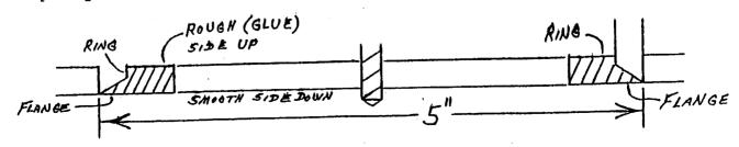
Note: If you do not have a circle cutter, you may use a scroll (jig) saw for cutting out the ring and the holes in the plates. A sanding drum would help smooth the holes but is not critical.
