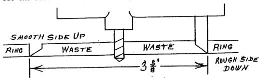
(c) Second, turn the remaining masonite over, rough side up, and reclamp after recentering the opening with the circle cutter; then cut through, leaving the special ring.
