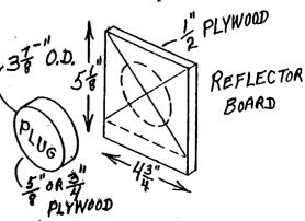
Note: Make the face board as shown. When you have cut out the hole and notch on the "holder" board, you <u>must</u> try it on the end of the pipe for size and make any further adjustments for a reasonably tight fit. Only <u>after</u> you are satisfied with the fit, do you pressure glue the face and holder boards together to complete the speaker end plate. Now match up the speaker plate (without the speaker attached) with the speaker end plate to drill the four 3/16" bolt holes.
