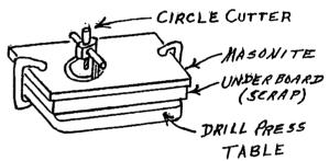
(b) First, cut out the center hole (3 5/8" dia.).
