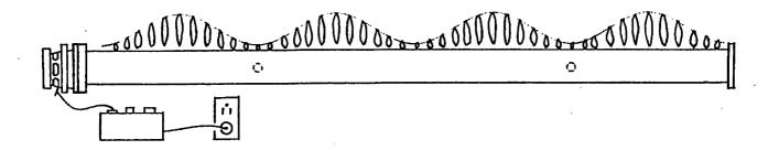
The single speaker flame tube is one of the most dramatic and educational pieces of physics demonstration apparatus ever developed. It is safe if used properly. It is relatively easy to build, inexpensive, and easy to operate.
