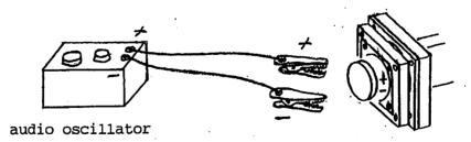
(b) "Beats" with a one-speaker flame tube. (VMI-Johnston design) Turn down the gas supply (keep flames low); may need to turn up the volume a little. Keep frequency low (long wavelength). Need two 100-ohm resistors (from Radio Shack?).
