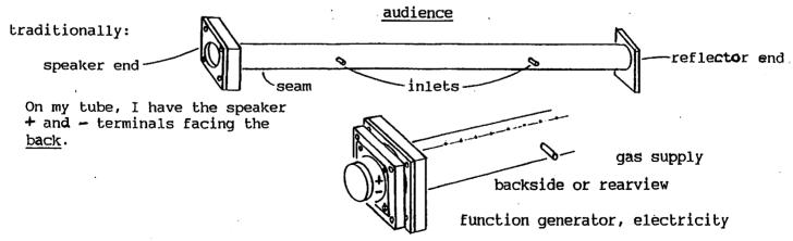
Notes: When attaching the end plates, attach the speaker plate <u>first</u> so the pipe's seam is on the bottom; drill the pilot holes with the angle driver and twist in the screws. Don't over-twist the screws and tear out the wood's "treads" - plywood is "soft"! The difficult part is finding a long, even place on a tabletop or floor (wall?), so the reflector (plug) end plate can be properly aligned with the speaker plate (won't wobble too much when used).
