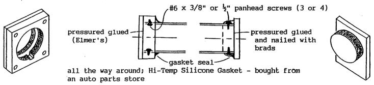
Notes: To fasten the speaker end plate, Philips head screws should be driven <u>inside</u>
