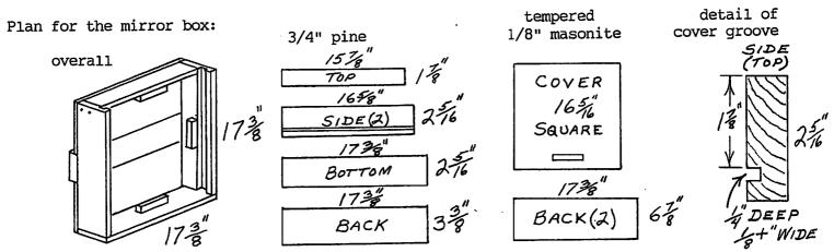
Assembly of mirror box: (a) Cut out the pine boards for the top, sides(2), bottom, and back. Cut the grooves for the cover in the side boards. TEST!
